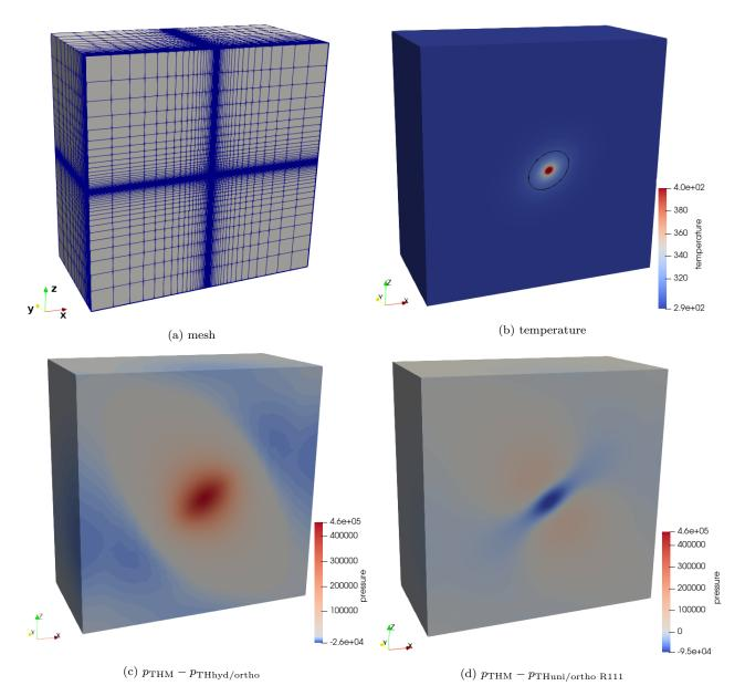
Figure 7: Mesh of orthotropic model (a) and temperature [T] = K, the black ellipse indicates the  $T_0 + 10 \text{ K}$  isosurface (b) pore pressure error  $[\Delta p] = \text{Pa of THhyd/ortho}$  (c) and pore pressure error  $[\Delta p] = \text{Pa of THuni/ortho}$  (d) with respect to the pore pressure of model THM at t = 5e6 s.
