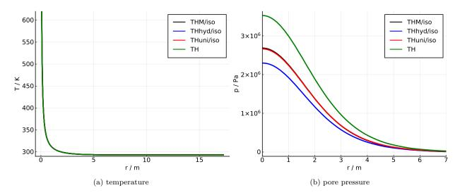
Figure 2: Temperature (a) and pore pressure (b) solution of a coupled THM point heat source problem in an isotropic medium along a diagonal line (1,1,1) extending radially away from the heat source. Solution given at time  $t = 5 \cdot 10^6$  s, i.e. about t = 57.9 d.
