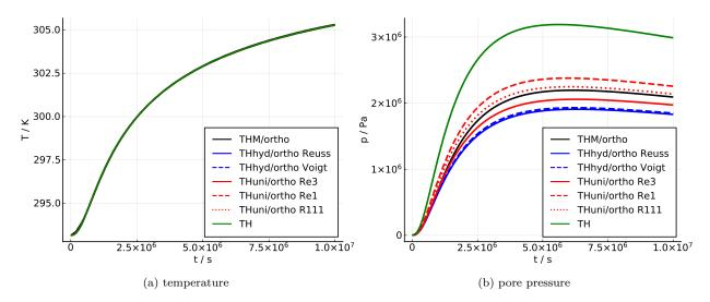
Figure 6: Temperature (a) and pore pressure (b) solution versus time of a coupled THM point heat source problem in an anisotropic medium at point P=(1.06, 1.06, 1.06) m.
