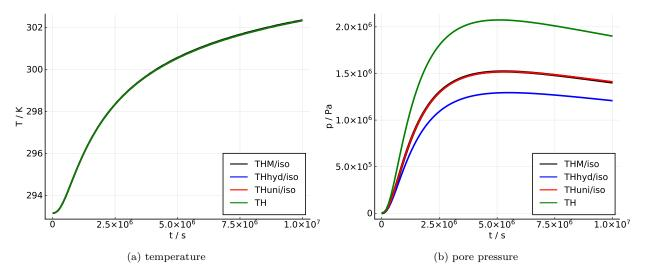
Figure 3: Temperature (a) and pore pressure (b) solution of a coupled THM point heat source problem in an isotropic medium versus time at point P=(1.06, 1.06, 1.06) m.
