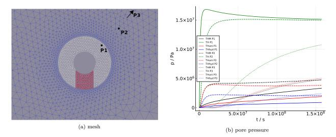
Figure 8: Mesh of the model domain consisting of three material groups (a) and pore pressure (b) solution versus time of a coupled THM cylindical heat source problem in an anisotropic medium for three points, one within the bentonite domain P1=(0.8, 0.8, 0.0) m and two points within the clay domain P2=(1.5, 1.5, 0.0) m. and P3=(10.5, 10.5, 0.0) m
