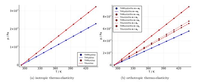
Figure 1: Exact correspondence between THM and TH models for given temperature increase and mechanical boundary conditions corresponding to constant hydrostatic stress (iso) or uniaxial strain (uni). Pressure response for isotropic (a) and orthotropic thermo-elasticity with three different orientations (b).
