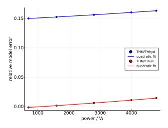
Figure 4: Time averaged model error at point P=(1.06, 1.06, 1.06) m versus heat source power.
