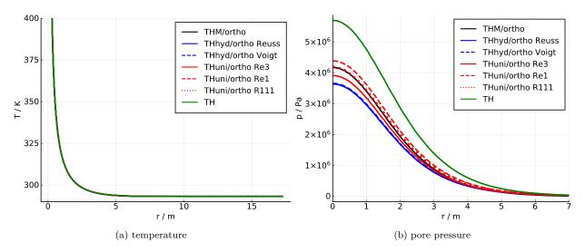
Figure 5: Temperature (a) and pore pressure (b) solution of a coupled THM point heat source problem in an anisotropic medium along the diagonal (1,1,1) extending radially outward from the heat source at time t = 5e6 s.
