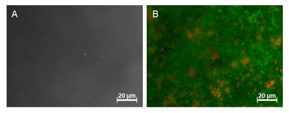
**Figure 3.** Comparison between the pictures obtained using optical microscope from: A) a new WE cleaned with sandpaper and B the WEs of one of the triplicate bioelectrochemical systems (BES2), treated with the nucleic acid staining kit LIVE/DEAD® BacLight<sup>™</sup> Bacterial Viability Kit (see Figure SI-4 for the rest of the data).
