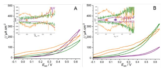
**Figure 2**: Representative CVs (scan rate of 1 mV s<sup>-1</sup>) and the respective 1<sup>st</sup> derivative (inset) using the cells (yellow), the WE/biofilm (purple) and the supernatant (green) of one of the triplicated bioelectrochemical system (BES1) at the end of the 1<sup>st</sup> (A) and of the 4<sup>th</sup> (B) batch cycles (see the data of the other replicates in Figure SI-2). The asterisk indicates the formal potential of the EET.
