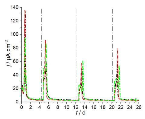
**Figure 1:** Current density ( $\mu$ A cm<sup>-2</sup>) of glucose fed bioelectrochemical systems (BES) inoculated with mouse feces polarized at +0.2 V vs. Ag/ AgCl sat. KCl (30 °C and 120 rpm) for four batch cycles (the gray vertical dotted lines indicate the starting of each cycle). The color of the traces refers to the three independent replicates: red for BES1, black for BES2 and green for BES3.
