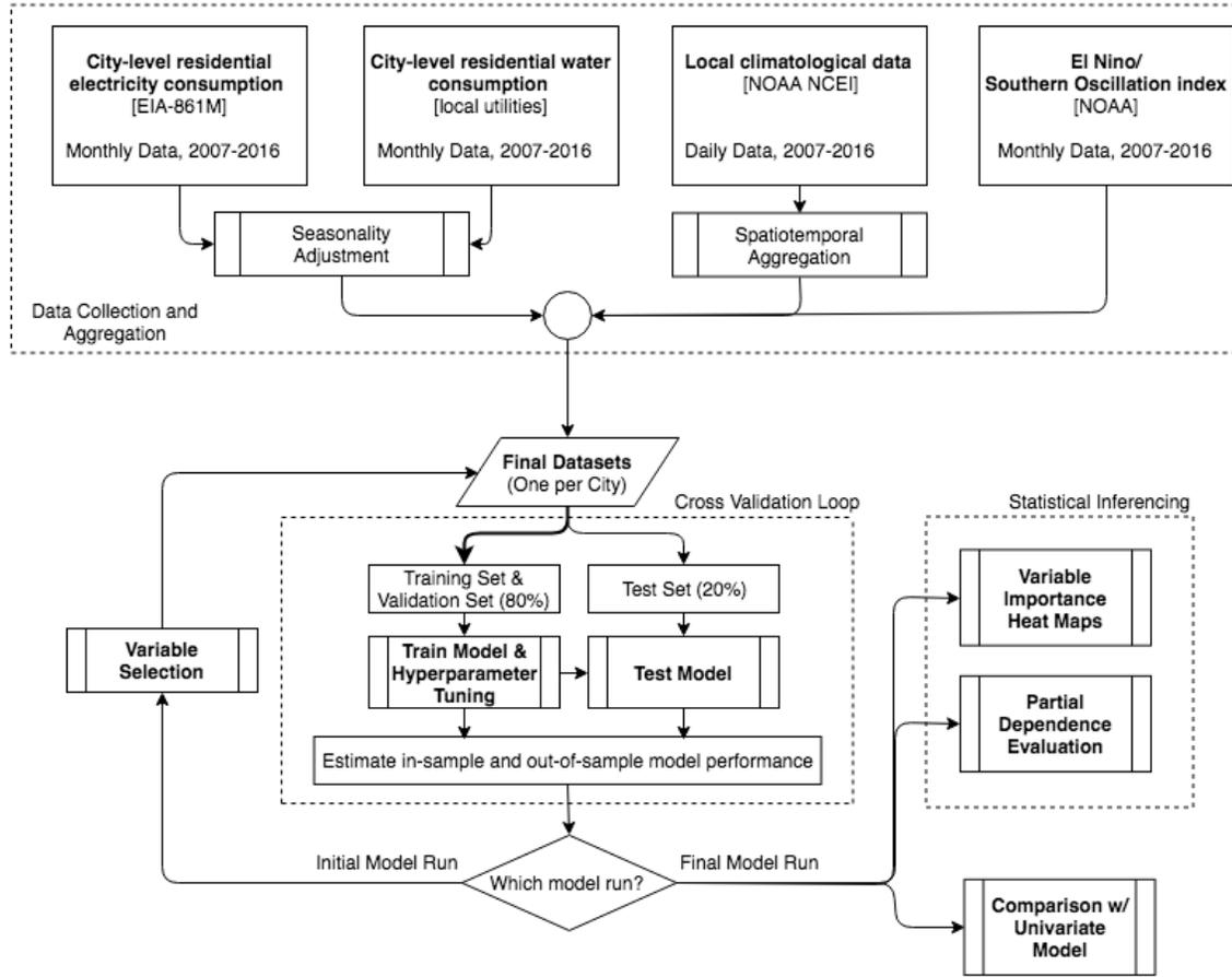
Figure 2: Schematic of the modeling process.
