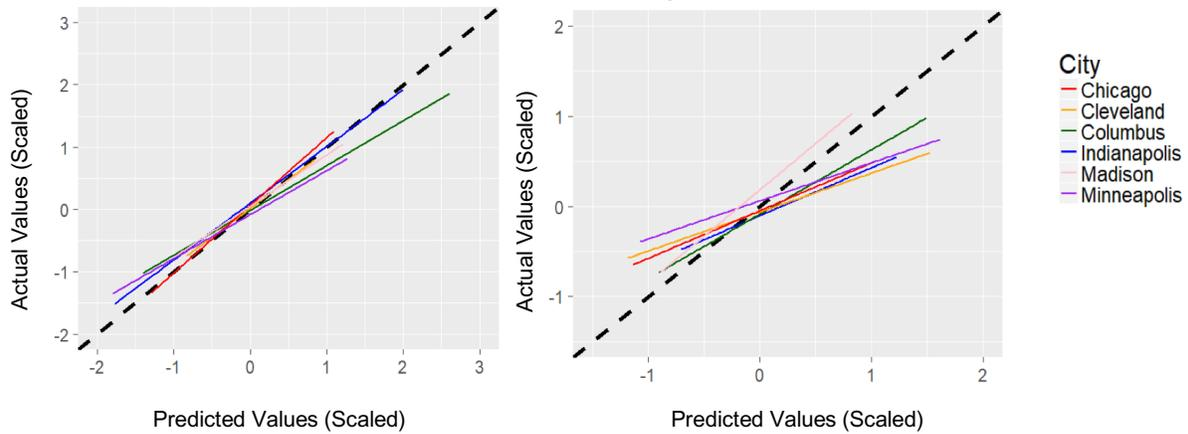
Figure 3: Out-of-sample model performance for (a) the original dataset (i.e., the dataset with seasonality) and (b) the seasonally adjusted dataset with the multivariate model. The response variables, water and electricity use, have been scaled to account for different units of measurement. The lines are best fit lines plotted through the predicted versus actual points, with a 45° dashed line for reference.
