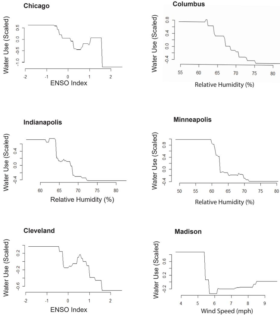
53 Figure 5: Partial dependence plots between the most important predictor variable and water use in each city. Note that the
