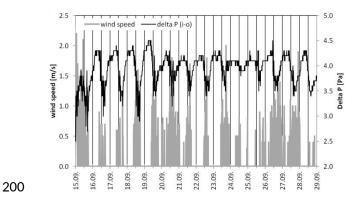
Fig. 5: Exemplary time series (2 weeks) of wind speed and indoor-outdoor pressure gradient
