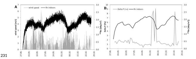
Fig. 7: Indoor radon concentrations (10 min values as recorded) and (7A) wind speed time series (10 min values as recorded) and (7B) pressure gradients (averaged day values) over the complete runtime of the experiment. Increased negative pressure indoors that is triggered by a higher wind speed results in a pressure induced "breathing" of the container.
