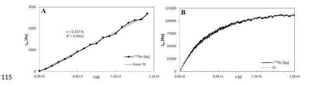
Fig. 1: Source calibration datasets "radon inventory vs. time" revealing an exhalation rate of  $F_{slope} = 0.26$  Bq/s based on the initial slope (1A) and an exhalation rate of  $F_{eq} = 0.24$  Bq/s based on the steady state inventory ( $I_{Rn} = 114$  kBq; 1B)
