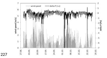
Fig. 6: Wind speed and indoor/outdoor pressure difference time series over the completeruntime of the experiment
