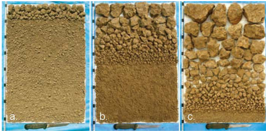
Figure 2: Visual key for scoring soil structure after a drop-shatter test. (a) Good, (b) moderate, and (c) poor physical condition. Reprinted from Shepherd et al. (2008).
