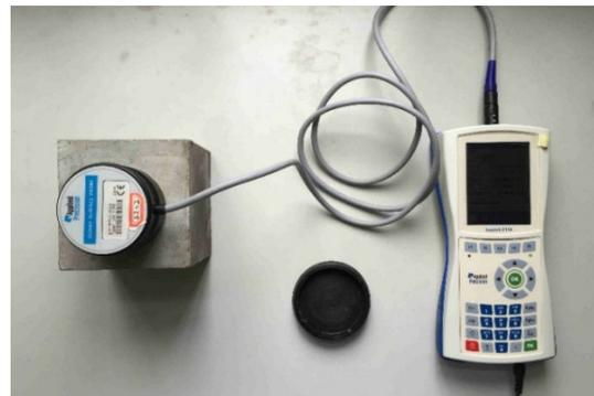
(b) Thermal conductivity measurement for hard rocks using a surface probe
