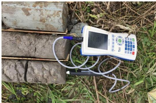
(a) Thermal conductivity measurement for soft soils using a needle probe
