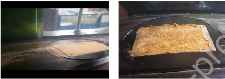
**Fig. 9: Erodibility tests.** Biofilm-sediment complex is exposed to increasing shear stress in the erosion flume SETEG (Strömungskanal zur Ermittlung der tiefenabhängigen Erosionsstabilität von Gewässersedimenten). Left is the bare sand that acts as the control (critical shear stress: 0.3 Pa), right is the mature biofilm after 6 weeks of growth (critical shear stress: 12 Pa after failure at the edges). Please see also S1 and S2 videos in the supplementary material.
