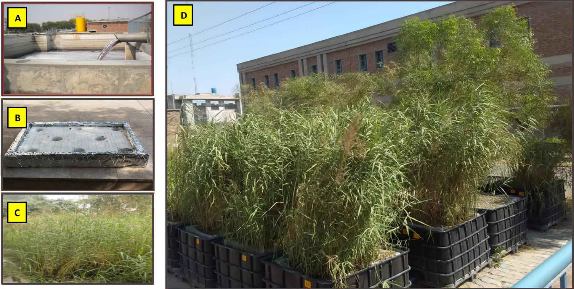
Fig. 1. Development and implementation of floating treatment wetlands (FTWs) macrocosms for the remediation of wastewater at Interloop Limited Khurrianwala, Faisalabad. Wastewater equalization tank (A), floating mat for the plantation of *Phragmites australis* seedlings (B), nursery of *P. australis* in the vicinity of NIBGE, Faisalabad (C), and growth of *P. australis* in FTWs macrocosms at the end of experimentation (D).
