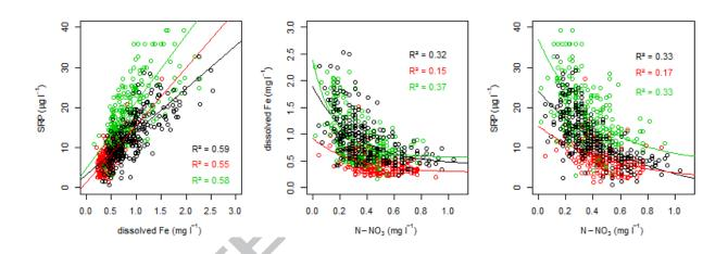
Figure 3: Concentration-concentration relationships between pairs of solutes. The relationship between SRP and dissolved iron was fitted with a linear model  $y = a+b^*x$ , and the relationship between NO3 and dissolved Fe and between NO3 and SRP was fitted with an exponential model  $y = a+b^*exp(-c^*x)$ . Carlsfeld 1 in black, Carlsfeld 2 in red, Carlsfeld 3 in green.
