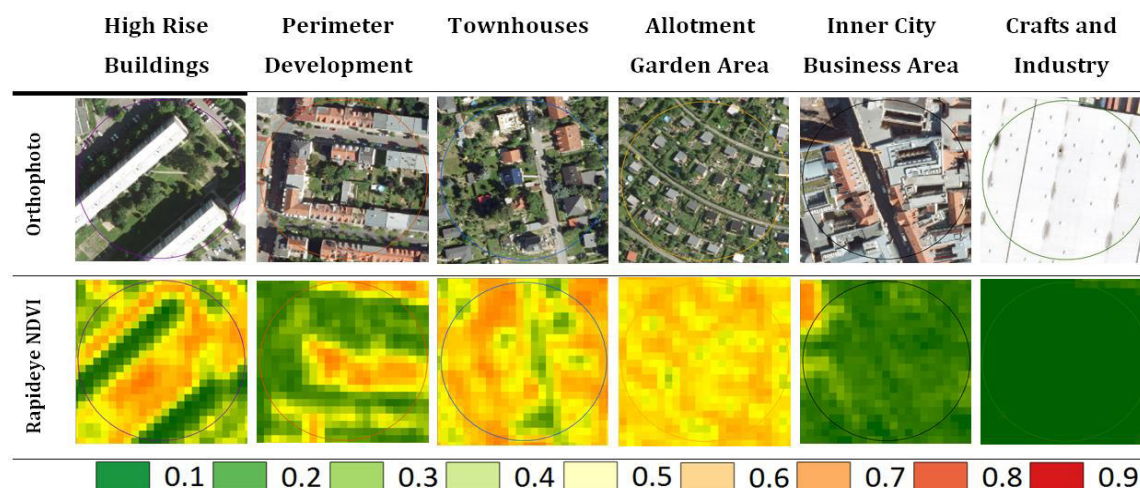
Fig. 6 Orthophoto and the corresponding NDVI values quantified by RapidEye data for urban built land use classes
