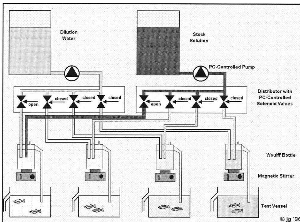
**Fig. 1. Schematic illustration of the setup of flow-through system for the life cycle study as conducted with EE<sub>2</sub> (17 $\alpha$ -ethinylestradiol) at the Fraunhofer Institute Schmallenberg**
