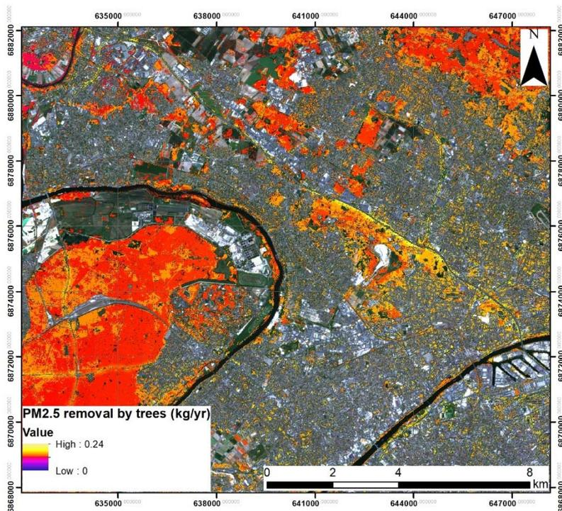
Figure 11: Modelled PM<sub>2.5</sub> removal by trees, with deciduous and evergreen types differentiated, overlaid on satellite imagery.
