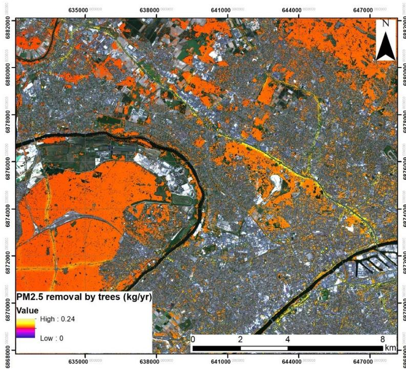
Figure 10: Modelled PM<sub>2.5</sub> removal by trees, with deciduous and evergreen types not differentiated, overlaid on satellite imagery.
