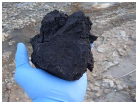
Figure 1: Oil sands are unconventional petroleum deposits and contain naturally occurring mixtures of sand, clay, water, and a dense and extremely viscous form of petroleum (bitumen). photo: N. Gerner, UFZ
