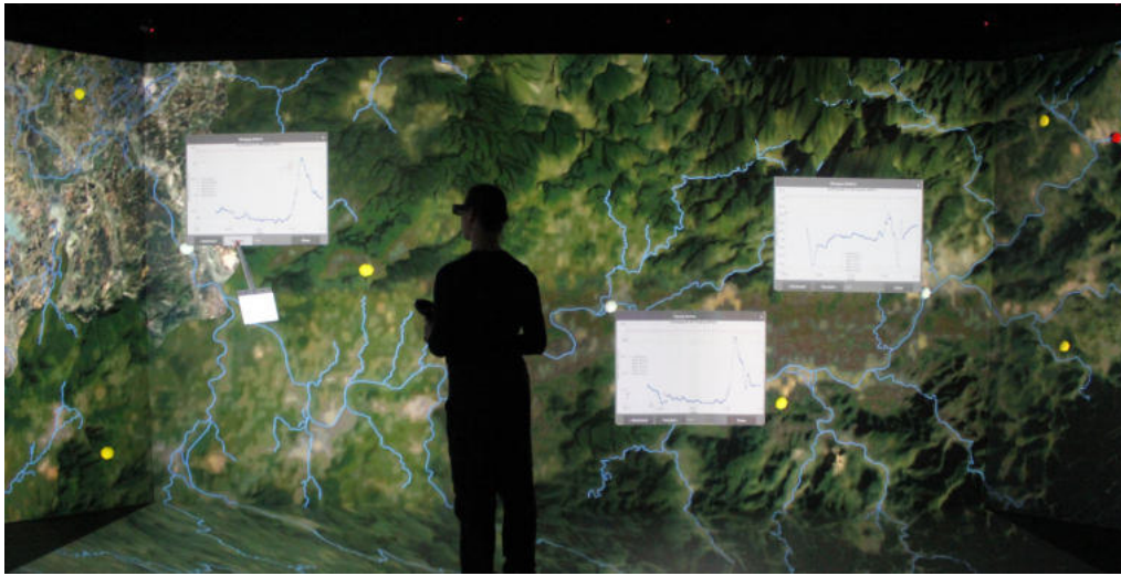
Figure 4: Practical use of the Virtual Reality environment: The user has zoomed in on the Xin River catchment with the river and its tributaries visualised in light blue. Flood hydrographs linked to gauging stations upstream, midstream and downstream (all marked in white) have been opened for further analysis.
