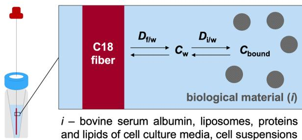
**Figure 1.** C18 SPME fiber experiments.  $C_w$  and  $C_{\text{bound}}$  are the freely dissolved and bound concentration of the test chemicals,  $D_{f/w}$  and  $D_{i/w}$  denote the distribution ratio between the fiber and water and between the tested biological material and water, respectively.
