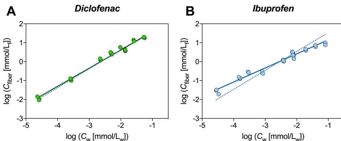
**Figure 3.** Fiber sorption isotherms of diclofenac and ibuprofen. The solid lines indicate the fitted Freundlich isotherms (eq. 4), the dotted lines show the fit with a fixed slope of 1 (eq. 4 with  $n_{Fr}=1$ ).
