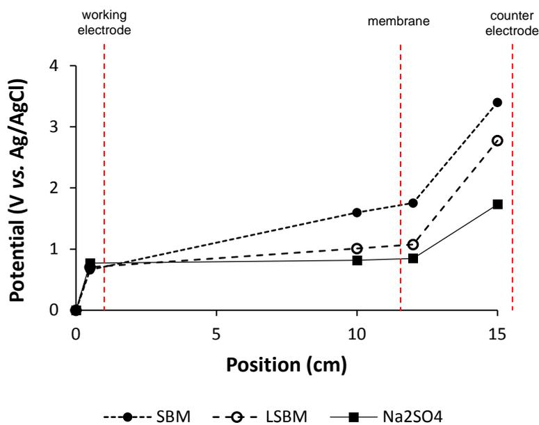
Figure 4: Electrochemical losses of the membrane (Nafion® 117) and different electrolytes (SBM, LSBM and 0.5 M Na<sub>2</sub>SO<sub>4</sub>) at a current density of 1.05 mA cm<sup>-2</sup> in the developed reactor assembly. Carbon fabric (129 cm<sup>2</sup>) contacted with a platinum wire (d=0.5 mm) was used as working and counter electrode.
