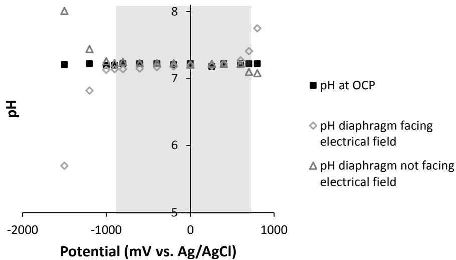
**Figure 6: pH values during an electrochemical measurement and at the open circuit potential (OCP) with different positions of the pH electrode diaphragm towards the electric field. Graphite sticks with surface area of 28.6 cm<sup>2</sup> were used as working and counter electrodes at varied potentials. Operating area is marked in grey.**
