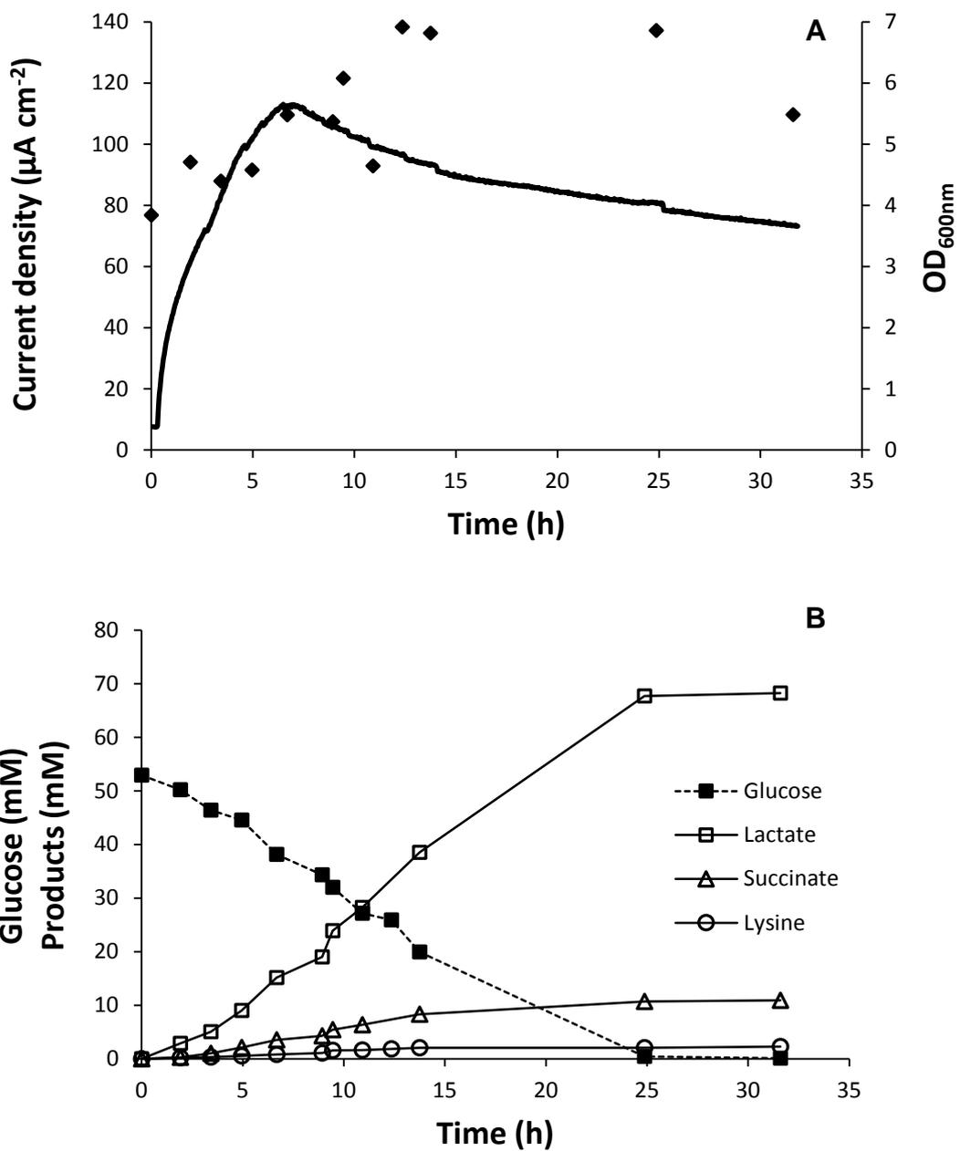
Figure 9: Electrochemically influenced conversion of glucose to lactate, succinate and lysine in *Corynebacterium glutamicum*. A: Current density (line) and  $\text{OD}_{600\text{nm}}$  (diamonds) during the conversion. B: Concentrations of the substrate glucose and the products lactate, succinate and lysine.
