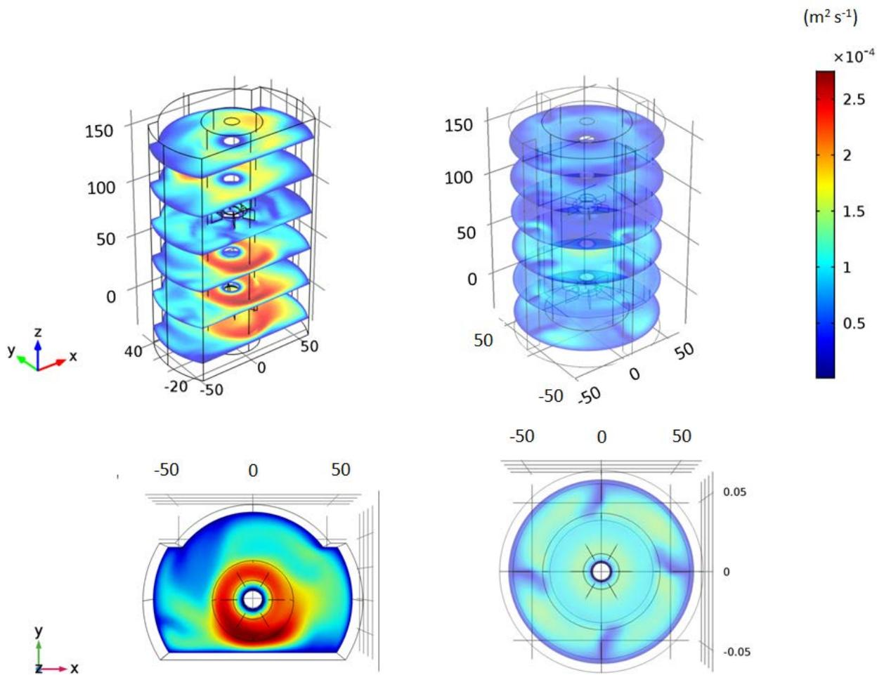
**Figure 5: Comparison of the turbulent kinematic viscosity in the bioreactor equipped with assembly 2 (left image) and a standard bioreactor (right image) simulated by computational fluid dynamics in COMSOL®. Dimensions in x, y and z direction are given in mm. The figures show slices in xy-planes at different heights throughout the different reactor configurations, with the magnitude of turbulent kinematic viscosity plotting on each slice.**
