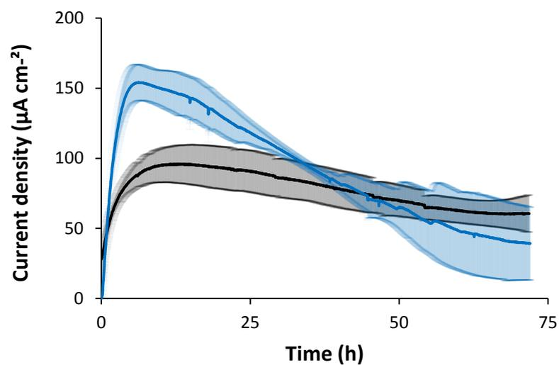
**Figure 7: Current production of  $12.5 \pm 2.8 \text{ mg L}^{-1}$  *S. oneidensis* in the separated (black) and non-separated (blue) electrobioreactor, respectively, using one layer of the working electrode carbon fabric poised at +400 mV vs. Ag/AgCl. The experiments were performed with repeats  $n = 3$  in the electrobioreactor with assembly 1 and assembly 2.**
