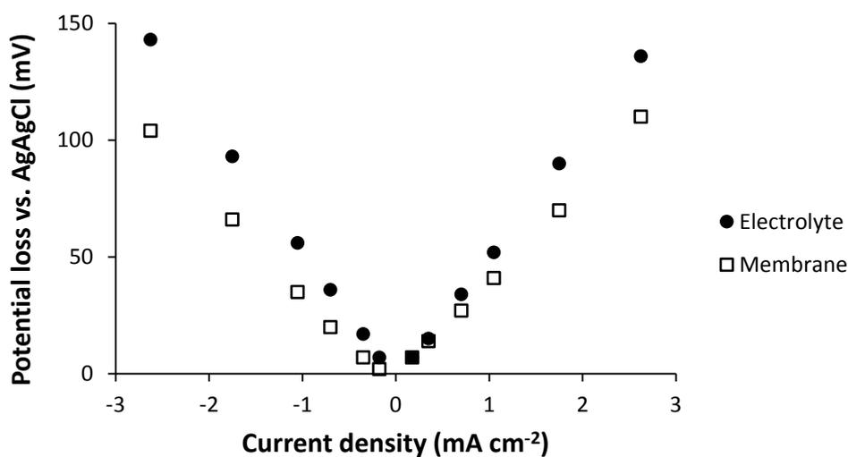
Figure 3: Electrochemical losses over the electrolyte 0.5 M Na<sub>2</sub>SO<sub>4</sub> and the membrane (Nafion® 117) in the developed reactor assembly 2. Graphite sticks with a surface area of 28.6 cm<sup>2</sup> were used as working and counter electrodes.
