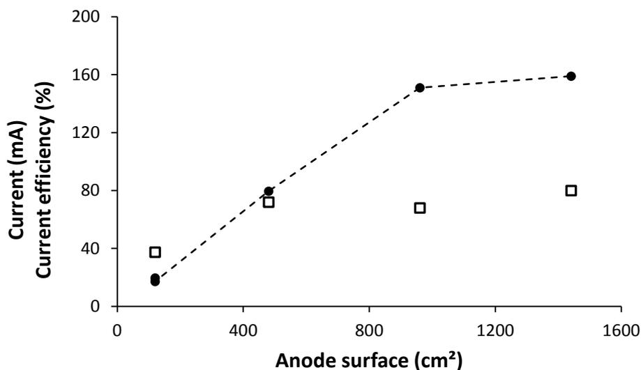
Figure 2: Closed dots show the maximum current productions of  $11.5 \pm 4.3$  mg/L *S. oneidensis* using assembly 1 having no separation between the working and counter electrode and using 1 to 12 layers (120 to 1440 cm<sup>2</sup> of carbon fabric) of the working electrode carbon fabric poised at +400 mV vs. Ag/AgCl. Open squares are the corresponding current efficiencies.
