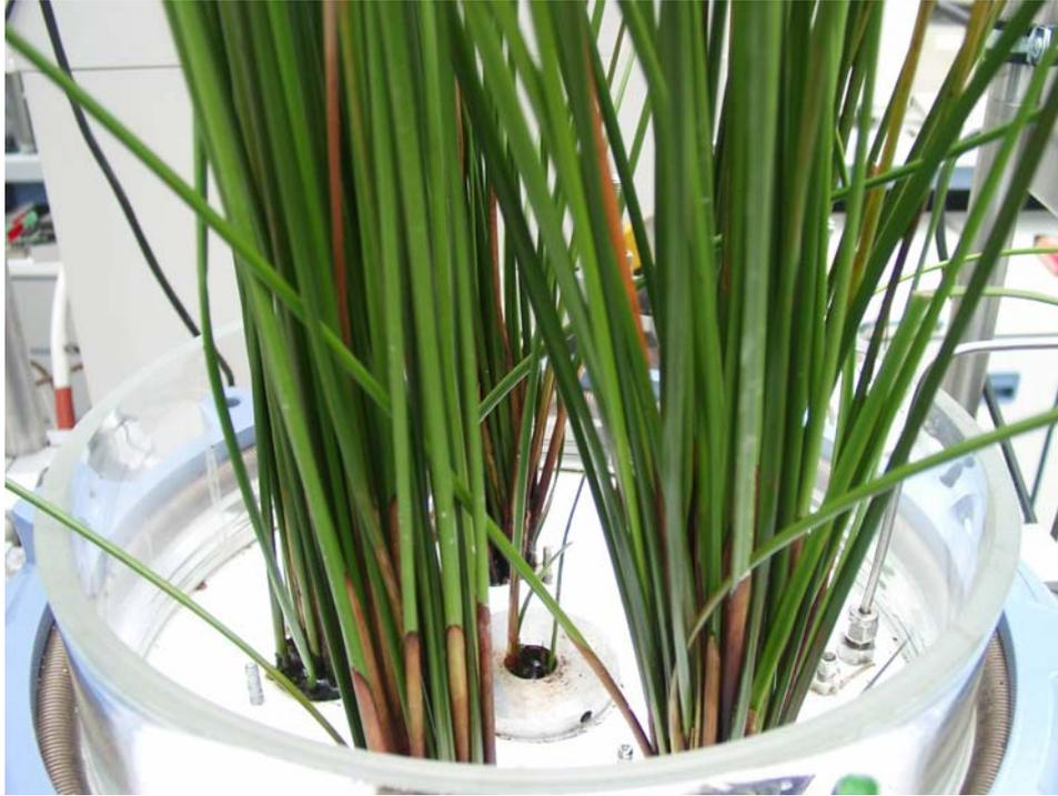
*Figure A3-2: Model rhizosphere reactors: Detail of the PTFE lid and plant openings containing Juncus effusus.*
