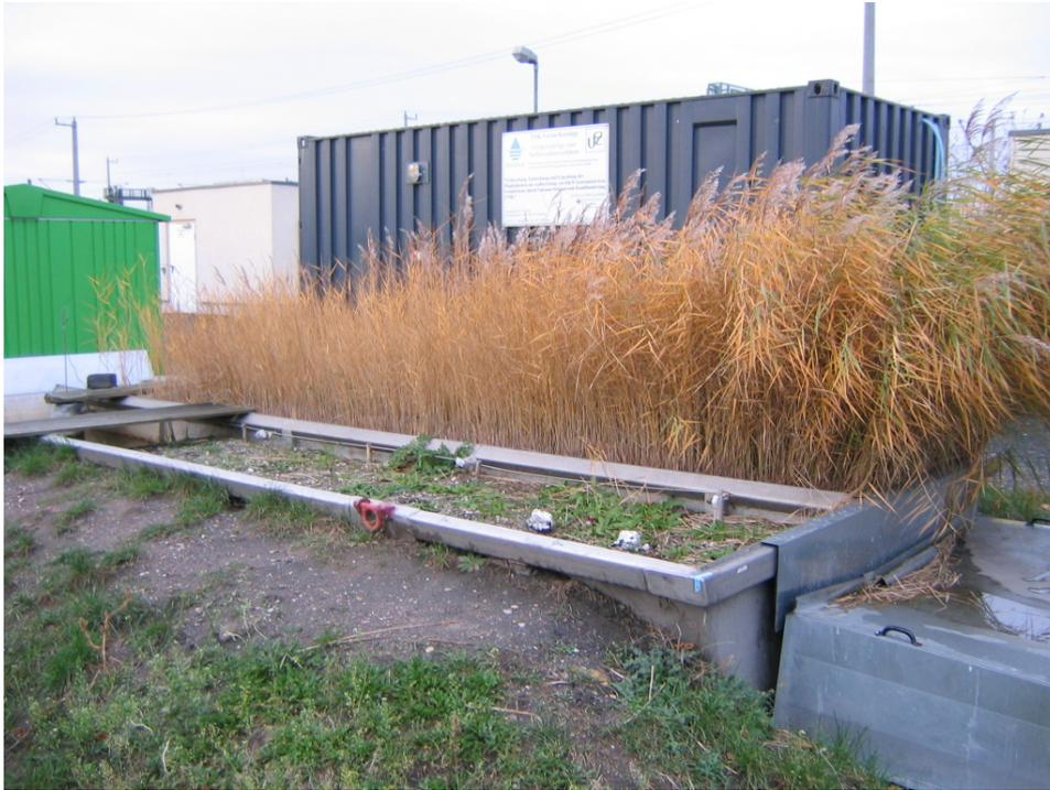
*Figure A2-2: Pilot-scale constructed wetland with dormant plants and unplanted reference systems in winter 2006.*
