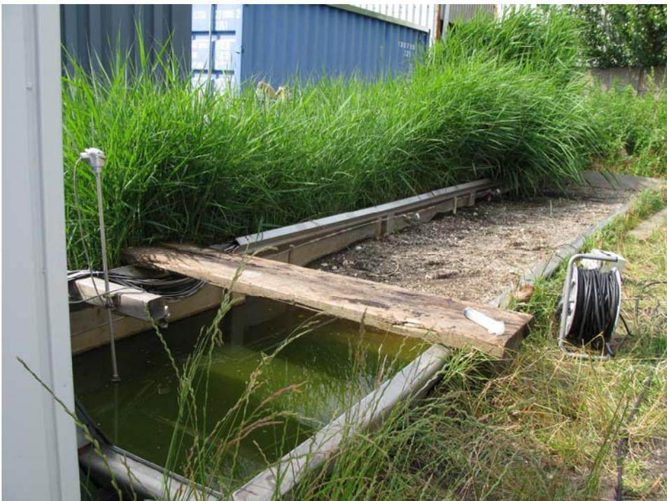
*Figure A2-3: Pilot-scale constructed wetland and unplanted reference systems in summer 2009; strong plant growth after fertilization.*
