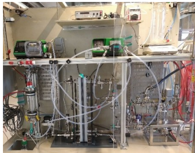
Figure 1. Photograph of the MEC breadboard including centrally the PVDF based MEC enabling steam sterilization
