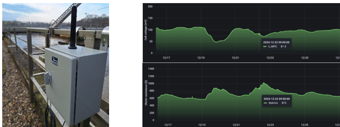
Figure 1: Picture of the installed embedded system (left) on the WWTP Ölbachtal (Ruhrverband, GER) and a representative screenshot of web interface (right).
