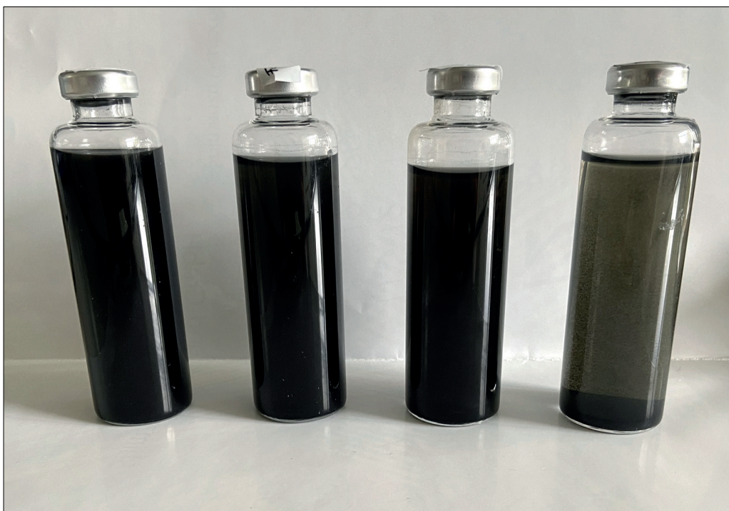
Figure S10 Aqueous suspensions (from left to right) of activated carbon spheres (aCS, [7], Fe/C 1/10, Fe/C 1/2 and freshly synthesized nZVI as described in [8] after 30 min of sedimentation; c_{\text{NaHCO}_3} = 10 \text{ mM} , c_{\text{particles}} = 1 \text{ g L}^{-1} , c_{\text{CMC}} = 10 \text{ mg L}^{-1} .
