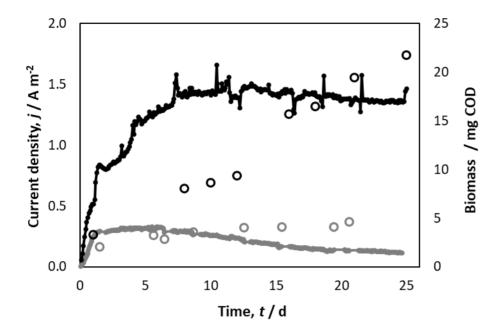
Figure 2 Time course of exemplary experiments showing current densities (lines) and corresponding biomass growth (circles). Experiments were performed with an acetate concentration of 0.5 mM at -0.2 V (grey, limiting conditions) and 5 mM at 0 V (black, non-limiting conditions).
