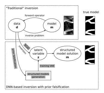
**Figure 6.** Adapted deep neural network-based (DNN) inversion scheme using a variational autoencoder (VAE) to represent complex geological structure in a latent space represented by sparse variable in which a stochastic gradient descent (SGD) can be applied to converge towards a more geologically realistic solution, modified from Lopez-Alvis et al. (2022).
