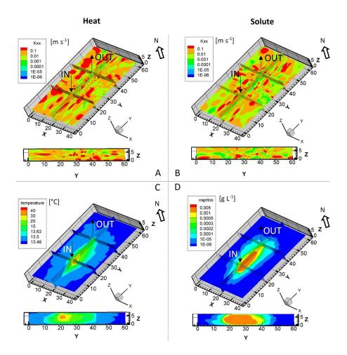
Figure 3. Hydraulic conductivity fields (a, b) and related simulations (c, d) obtained by inversion of temperature (a–c) and solute tracer concentration data (b–d) from heat and solute tracer experiments (modified from Hoffmann et al., 2019, Table 2A1).
