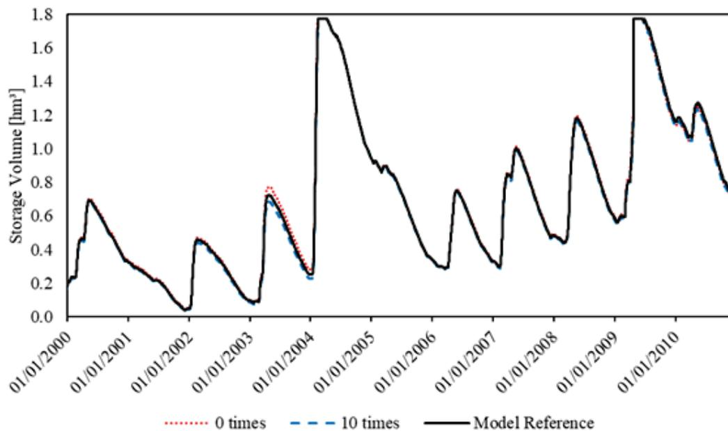
**Figure 15** Comparison for storage volumes in Do Coronel (2000 – 2010) with modifications in the dimensions of the small reservoirs in 0 and 10 times. “0 times” means the total absence of small reservoirs. “10 times” means a ten times increase in the parameters that represent the volumes of these small reservoirs. Model reference means the original parameterization.
