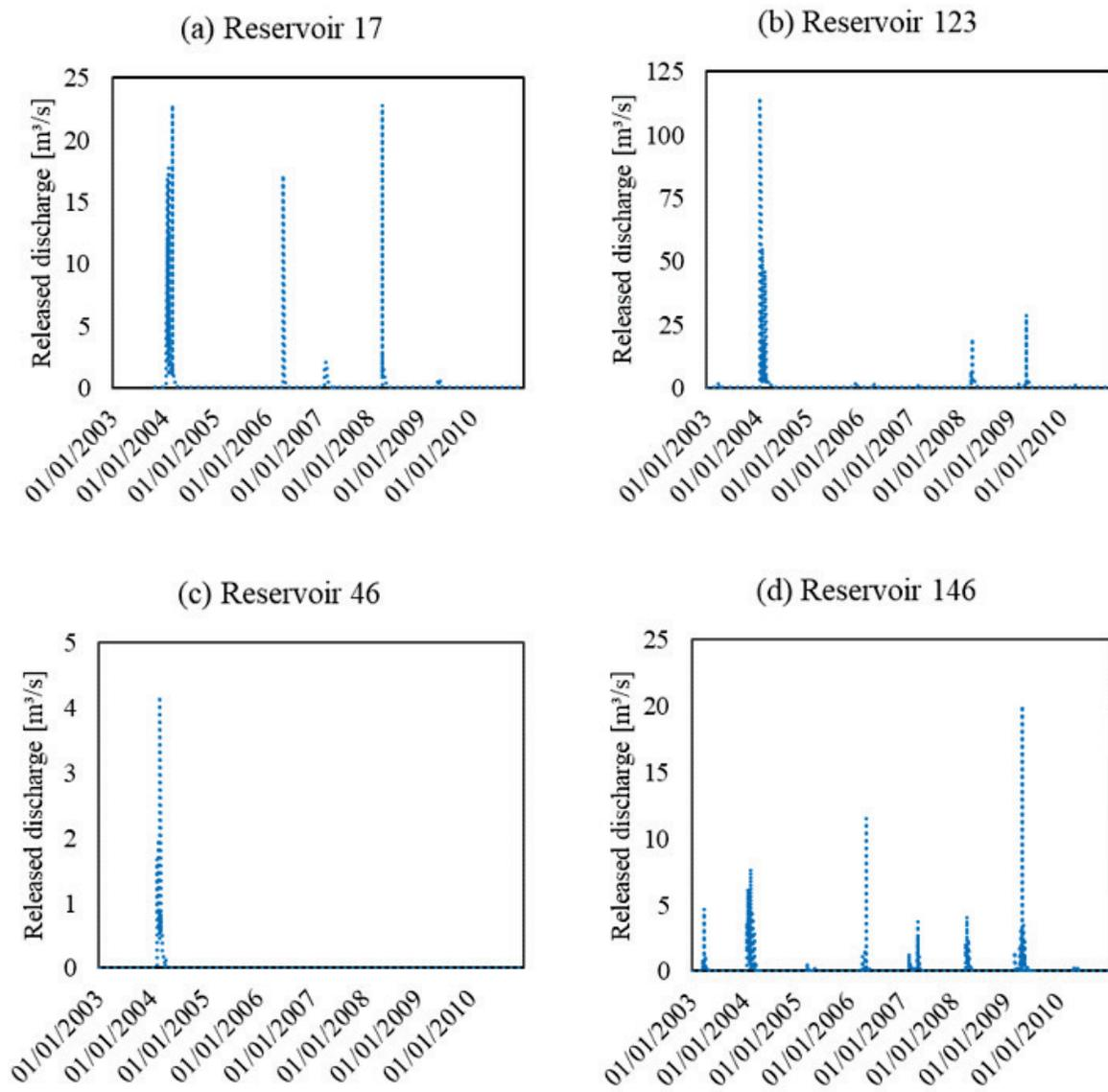
**Figure 10** Hydrographs for simulated daily discharges released from the private reservoirs No. 17 (a), No. 123 (b), No. 46 (c) and No. 146 (d) via spillway for the years 2003-2010.
