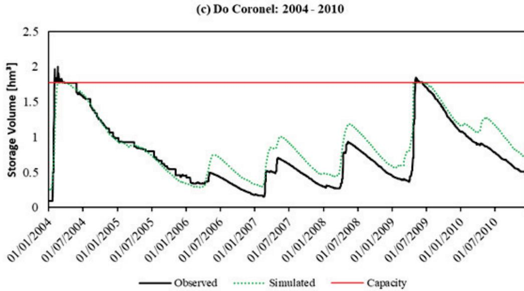
**Figure 8** Comparison of observed by state water agency and simulated by SWAT daily storage volumes in the three strategic reservoirs for the calibration and validation periods: (a) Poço da Pedra (storage capacity 52 hm<sup>3</sup>, simulation 1986 - 2010) (b) Benguê (storage capacity 19.56 hm<sup>3</sup>, simulation 2000 - 2010), (c) Do Coronel (storage capacity 1.77 hm<sup>3</sup>, simulation 2004 - 2010).
