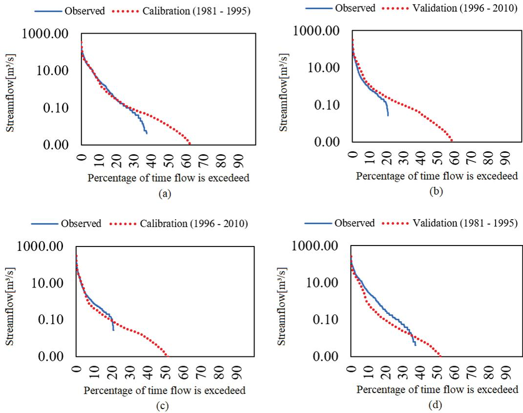
**Figure 6** Comparison of observed and simulated log flow duration curves for: (a) calibration in 1981 – 1995; (b) validation in 1986 – 2010; (c) calibration in 1986 – 2010; (d) validation in 1981 – 1995.
