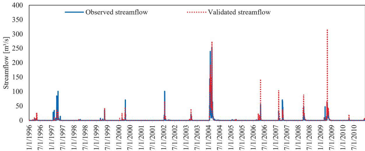
(c) Hydrograph for Malhada gauging station for the calibration period of 1996 - 2010
