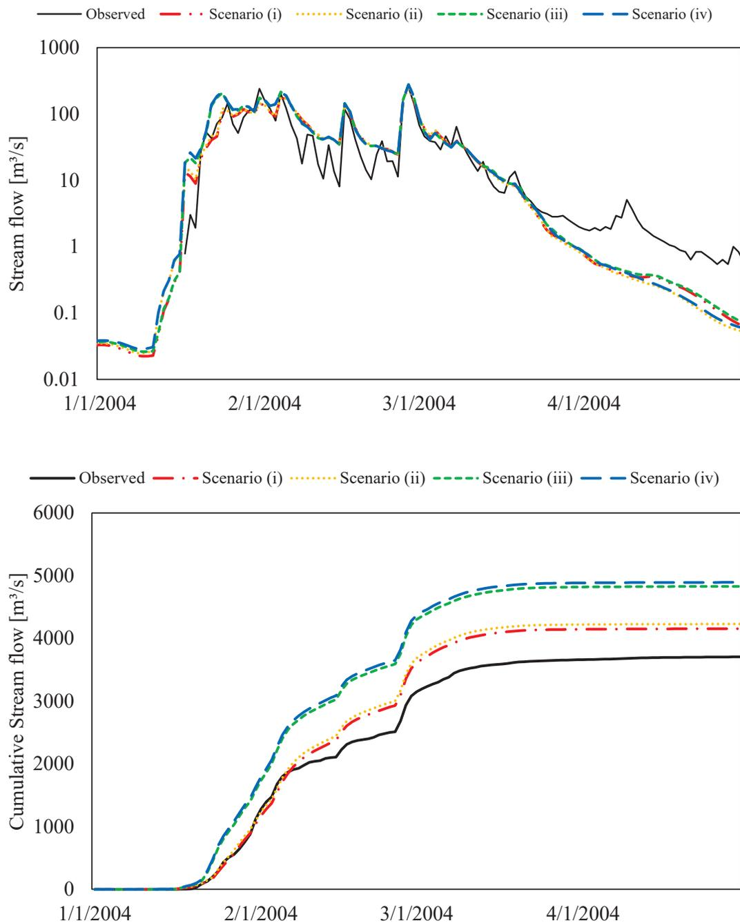
**Figure 11** Hydrographs and cumulative stream flow at Malhada station showing observed values and 4 scenarios of reservoirs during the year of 2004: scenario (i) considering all strategic reservoirs and small reservoirs (reference); (ii) removing all small reservoirs in the hydrological system, but keeping only the strategic reservoirs; (iii) removing all strategic reservoirs but keeping only the small reservoirs; (iv) removing all reservoirs.
