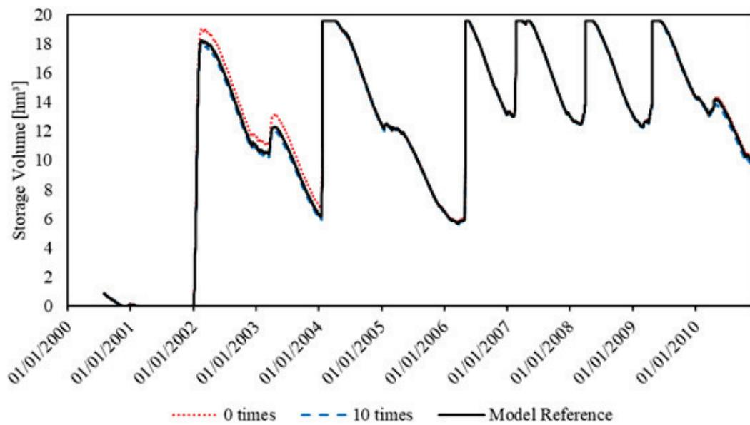
**Figure 14** Comparison for storage volumes in Benguê (2000 – 2010) with modifications in the dimensions of the small reservoirs in 0 and 10 times. “0 times” means the total absence of small reservoirs. “10 times” means a ten times increase in the parameters that represent the volumes of these small reservoirs. Model reference means the original parameterization.
