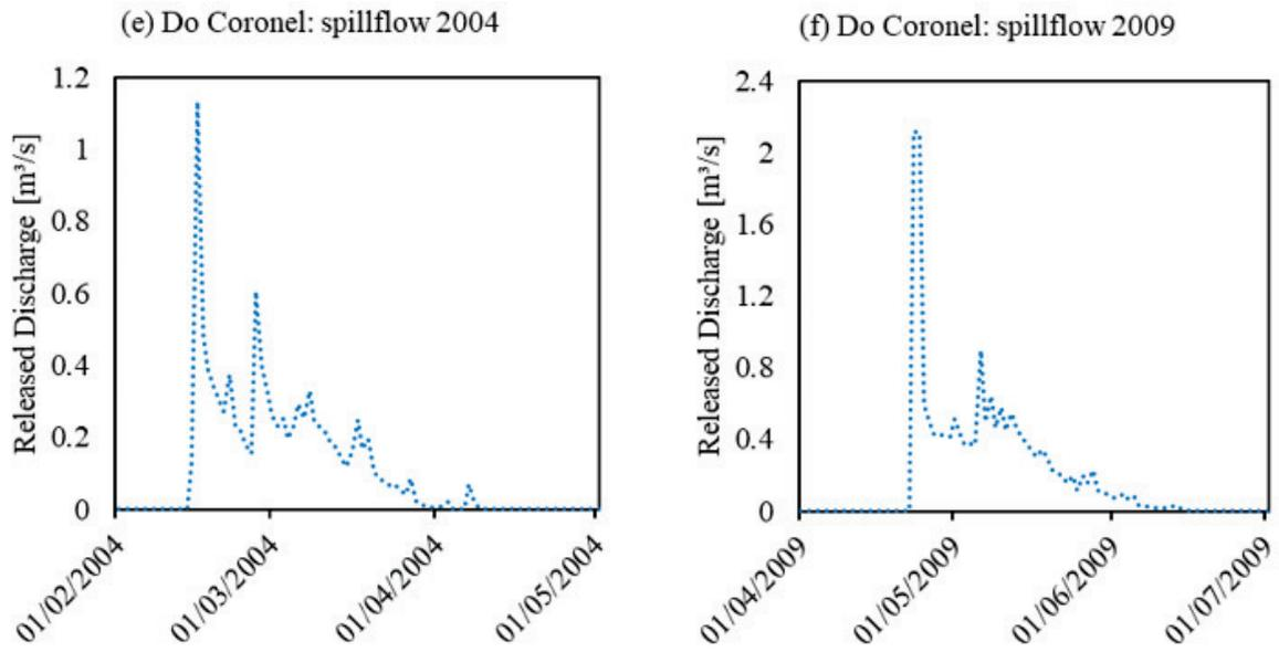
**Figure 9** Hydrographs of released discharge for simulated outflow over the spillway of the three strategic reservoirs for model simulations: (a) Poço da Pedra – 2004; (b) Poço da Pedra – 1986; (c) Benguê – 2004; (d) Benguê – 2009; (e) Do Coronel – 2004; (f) Do Coronel – 2009.
