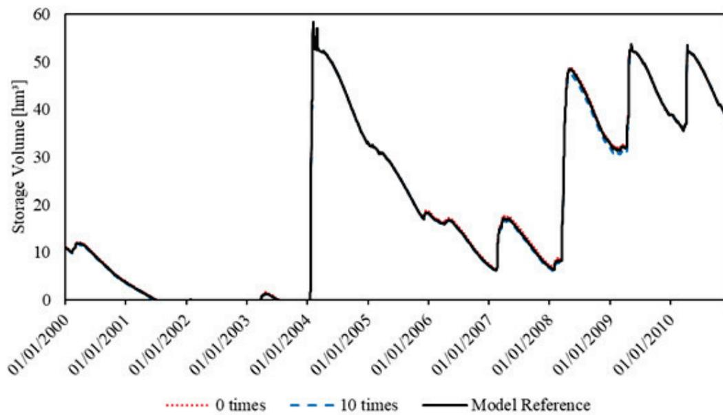
**Figure 13** Comparison for storage volumes in Poço da Pedra (2000 – 2010) with modifications in the dimensions of the small reservoirs in 0 and 10 times. “0 times” means the total absence of small reservoirs. “10 times” means a ten times increase in the parameters that represent the volumes of these small reservoirs. Model reference means the original parameterization.
