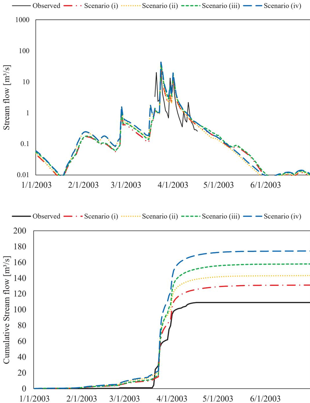
**Figure 12** Hydrographs and cumulative stream flow at Malhada station showing observed values and 4 scenarios of reservoirs during the year of 2003: scenario (i) considering all strategic reservoirs and small reservoirs (reference); (ii) removing all small reservoirs in the hydrological system, but keeping only the strategic reservoirs; (iii) removing all strategic reservoirs but keeping only the small reservoirs; (iv) removing all reservoirs.
