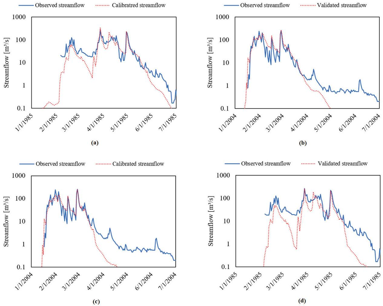
**Figure 7** Comparison of observed and simulated hydrograph for daily discharges at Malhada gauging station for: (a) calibration year of 1985; (b) validation year of 2004; (c) calibration year of 2004; (d) validation year of 1985.
