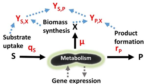
**Figure 1:** Quantitative physiology and performance characterization of whole-cell biocatalysts in biotechnology based on cell kinetics and yield coefficients.
