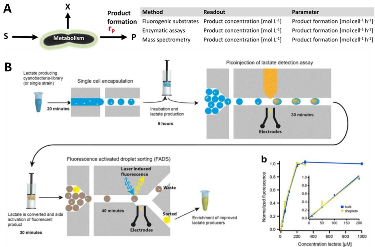
**Figure 5: A)** Analytical methods, readouts, and deducible kinetic parameters for product formation rates at a single-cell level. **B)** Quantifying lactate production by phototrophic cyanobacteria cultivated in microfluidic droplets via a pico-injected enzymatic assay [61].
