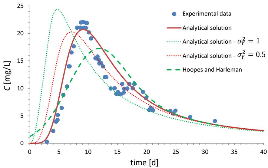
Figure 7: Experimental results of the dipole tracer test at the Mobile site and its interpretation by the proposed analytical model as well as the equivalent homogeneous solution of Hoopes and Harleman (1967); experimental data from Molz et al. (1986).
