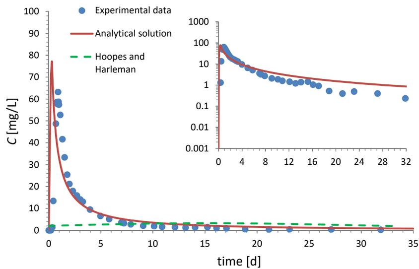
Figure 6: Experimental results of the dipole tracer test at the MADE site and its interpretation by the proposed analytical model as well as the equivalent homogeneous solution of Hoopes and Harleman (1967); experimental data from Bianchi et al. (2011).
