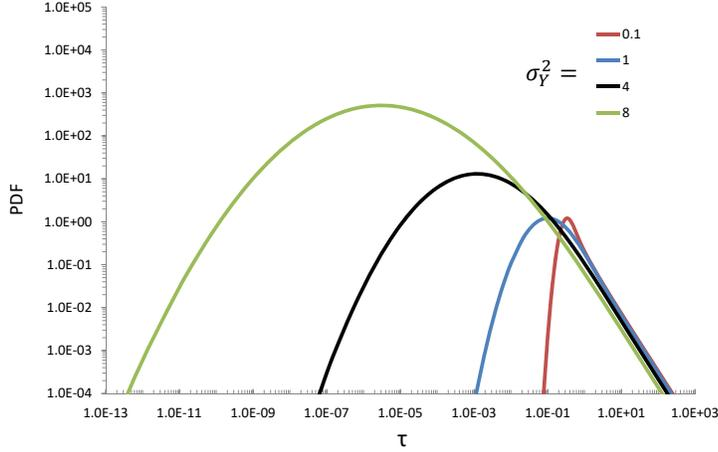
Figure 3: The travel time PDF  $f_{\tau}^F$  as function of the dimensionless travel time  $\tau = qt/(4\pi na^2)$  for a few values of the log-conductivity variance  $\sigma_Y^2$ .
