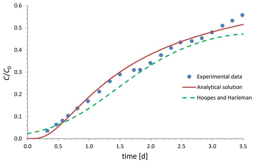
Figure 8: Experimental results of the dipole tracer test at the Barstow site and its interpretation by the proposed analytical model as well as the equivalent homogeneous solution of Hoopes and Harleman (1967); experimental data from Robson (1974).
