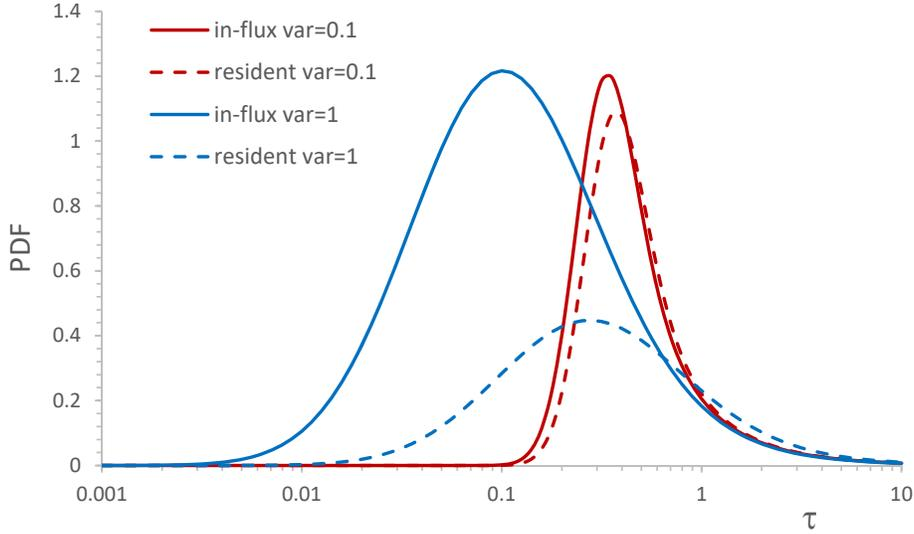
Figure 4: Comparison between the travel time PDFs pertaining to flux-proportional ("in-flux"; solid lines) and resident modes ("resident", dashed lines) injection conditions, for  $\sigma_Y^2 = 0.1$  (red lines) and  $\sigma_Y^2 = 1$  (blue lines).
