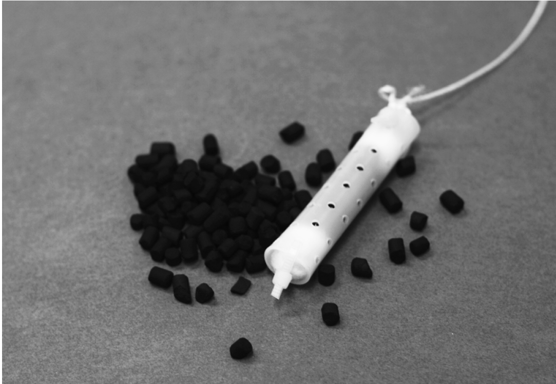
Fig. 8.2 - “Classical” BACTRAP probe with activated carbon matrix
