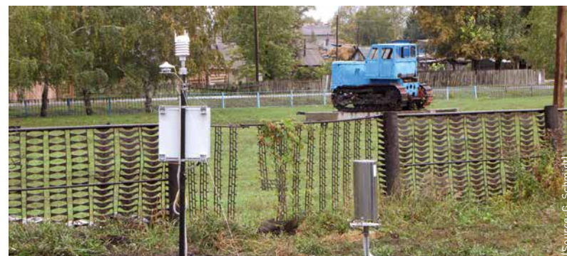
Climate and soil moisture measuring station in the Perwomaisk test area.
