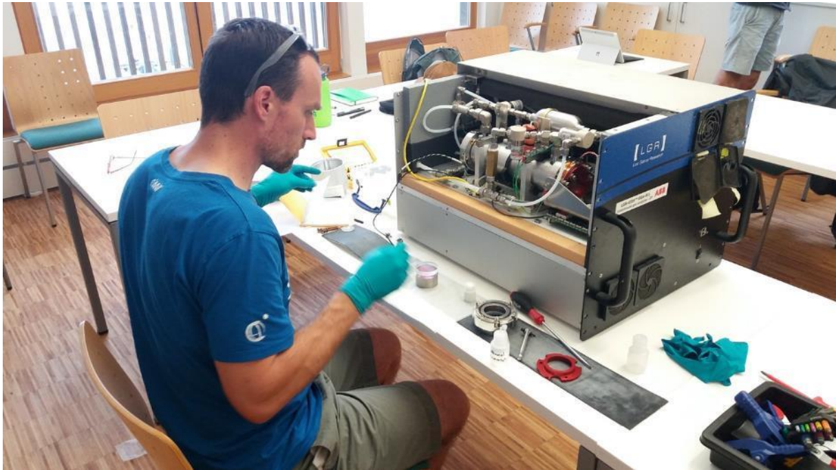
Fig. 5: Bill Cable Cleans the mirrors in a different Los Gatos Greenhouse Gas Analyzer that needed some maintenance. [Photo by Antje Eulenberg]
