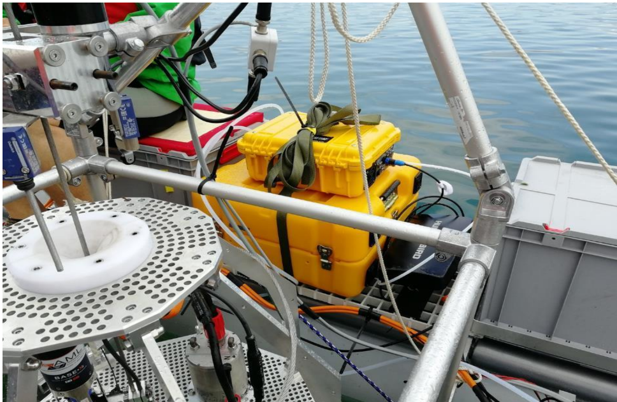
Fig. 4: The two yellow cases in this photo are the Dissolved Gas Extraction System (DGES, bottom) and Microportable Greenhouse Gas Analyzer (MGGA) from Los Gatos Research. In combination, these instruments extract CO 2 and Methane from water (DGES) and determine their concentration (MGGA). Here they are installed on SWOPpy, enabling automated measurements of Methane and CO 2 in the surface waters of the lake. [Photo by Anton Kuech]
