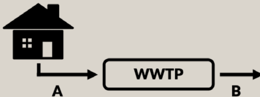
Figure 3 EN 12566-3. A: Influent; WWTP: Prefabricated wastewater treatment plant and B: Outflow Source: NICE, 2021).
