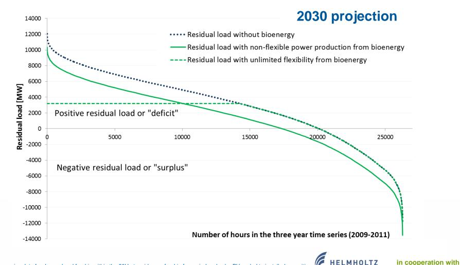
Data: time series data for demand and feed-in within the 50Hertz grid area; feed-in from wind and solar PV scaled to installed capacities expected for 2030 according to Leitstudie 2011. Flexible power generation from biomass modelled to minimize variances in residual load.
