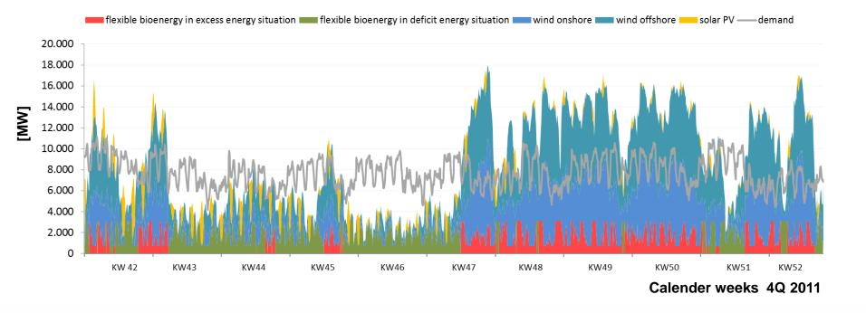
Data: time series data for demand and feed-in within the 50Hertz grid area; feed-in from wind and solar PV scaled to installed capacities expected for 2030 according to Leitstudie 2011 Flexible power generation from biomass modelled to minimize variances in residual load.
