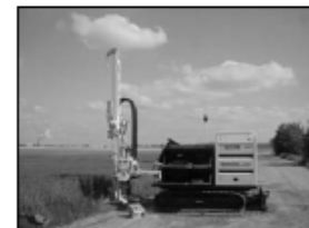
Fig. 9: Geoprobe ® Direct-Push unit during EC-logging
