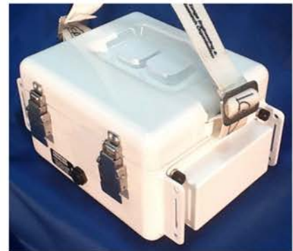
ZEN System Distributed Array Multi-function Receiver including 32-Bit Magnetotellurics
