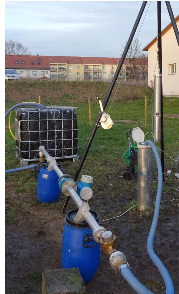
*Tracer test with 1000 liters of snowmelt at the groundwater test site in Pirna, Saxony*
