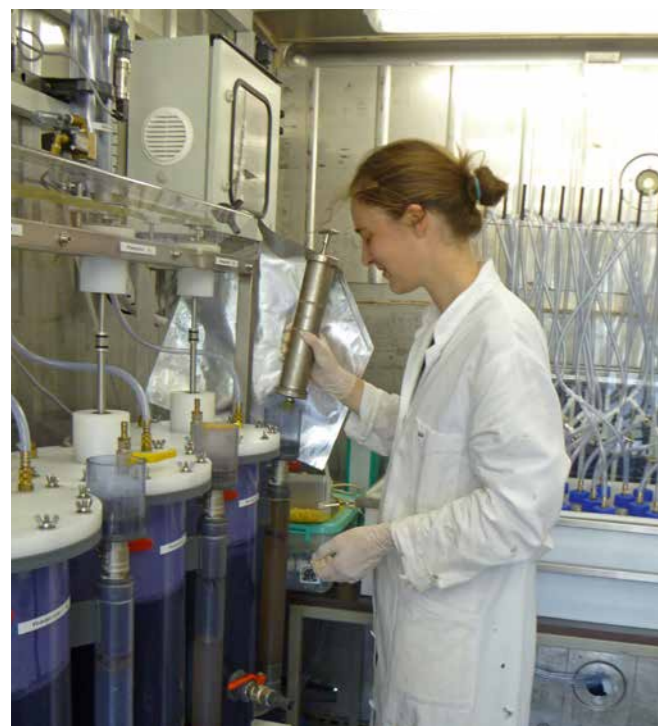
Fig. 37: Pass-through reactor for anaerobic sewage sludge – stabilization tests. → Photo: H. Feldhaus, TU Braunschweig
