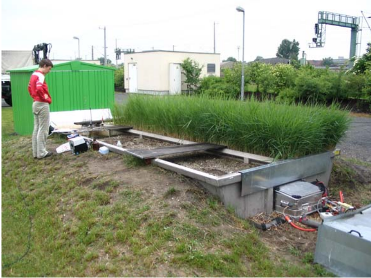
Figure 1: Constructed wetland for treatment of chlorobenzene contaminated groundwater in Bitterfeld
