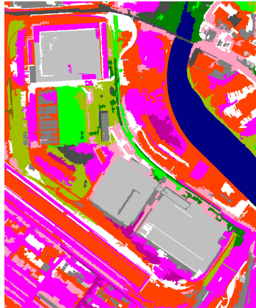
Figure 3. Classified image sample showing large industrial buildings (in light and dark grey), various numbers of cars on parking lots (in red, purple, and pink), impervious surface without distinction (in white) grass (in bright green), neglected sparse vegetation (in olive green).
