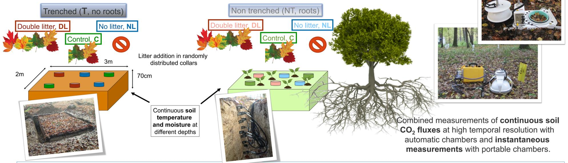
Combined measurements of **continuous soil CO<sub>2</sub> fluxes** at high temporal resolution with automatic chambers and **instantaneous measurements** with portable chambers.
