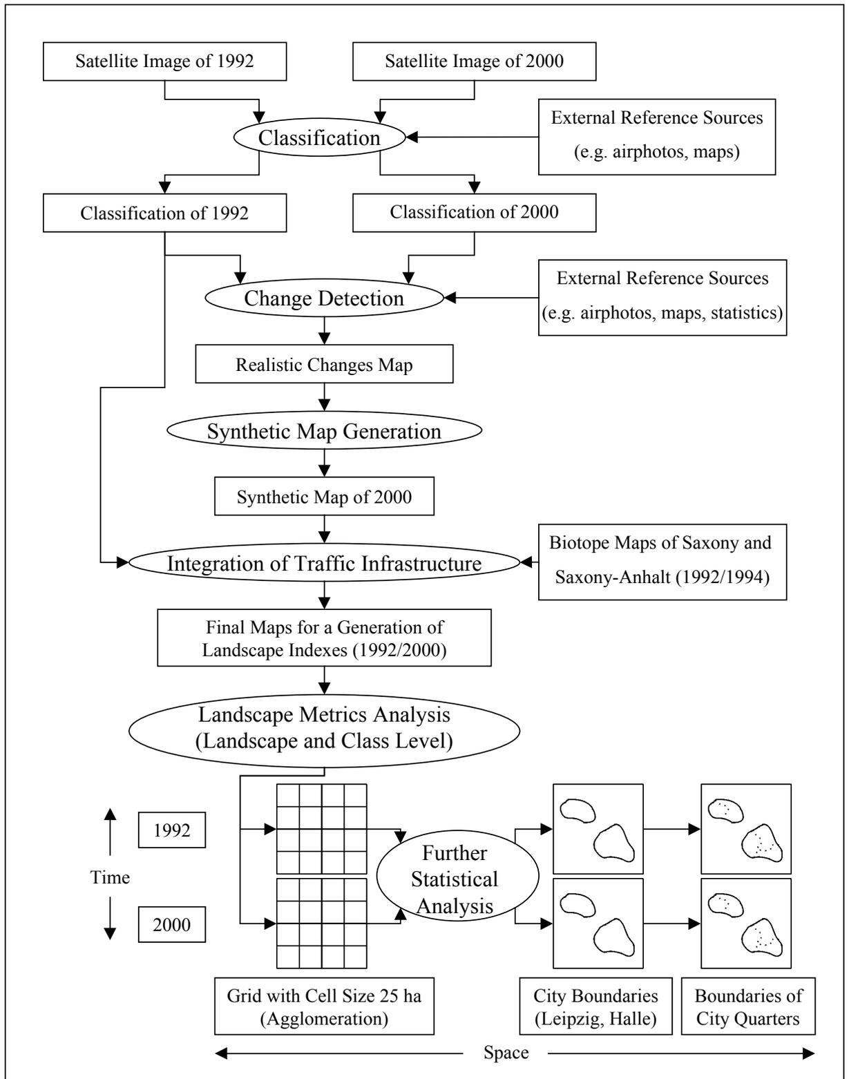
Figure 1: Structure of this work.
