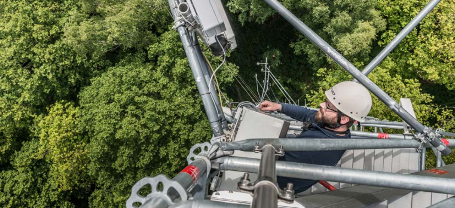
The 50 meter-high measuring tower in the Forest-Climate Observatory in Hohen Holz in Saxony-Anhalt is part of the TERENO observatory. Here scientists record numerous variables: climate data, greenhouse gases, data on vegetation, soils and the water budget.
