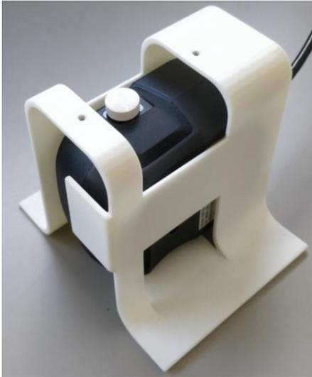
Put the device in the holder and place the tablet on the measurement window using tweezers
