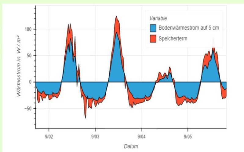
Figure 2 - **Composition of the soil heat flux at the surface:** Time series of the soil heat flux measured at a depth of 5 cm ( $Br$ ) and the determined soil heat flux at the surface  $B_0$ . The red areas denote the heat storage of the upper substrate layers.
