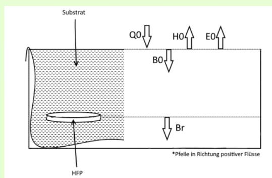
Figure 1 - **Energy balance on the green roof:** The main driving factor is the net radiation ( $Q_0$ ), which is partitioned into the latent heat flux ( $E_0$ ), sensible heat flux ( $H_0$ ) and soil heat flux ( $B_0$ ). The measurement of the soil heat flux in the substrate ( $Br$ ) can be performed by heat flux plates (HFP) in the substrate only at a reference depth. In general,  $B_0 \neq Br$ , as the layer between the two points stores energy.
