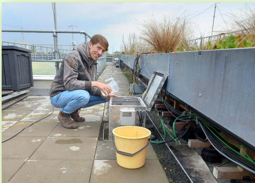
Figure 3: **Johannes Stüllein** calibrating roof runoff measurements.
