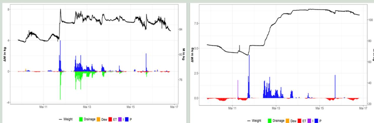
Figure 2: Weight of the substrate in the gravel (left) and wetland roof (right) with certain water exchange processes for the 19th calendar week of the year 2021: The water exchange processes are shown with a temporal resolution of 30 minutes via colored bars (blue=rainfall, purple=irrigation, green = runoff, orange= dewfall, red=evapotranspiration).
