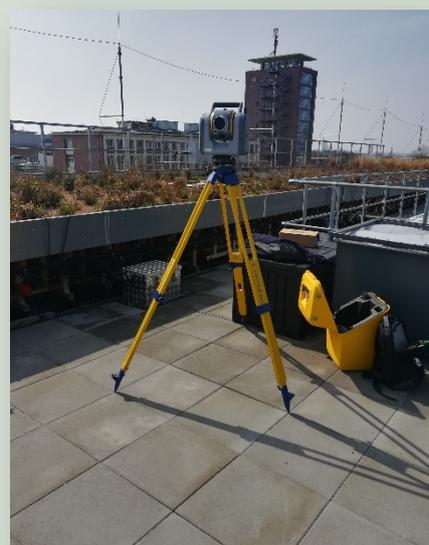
Figure 3: Trimble SX10 scanning total station on the research canopy
