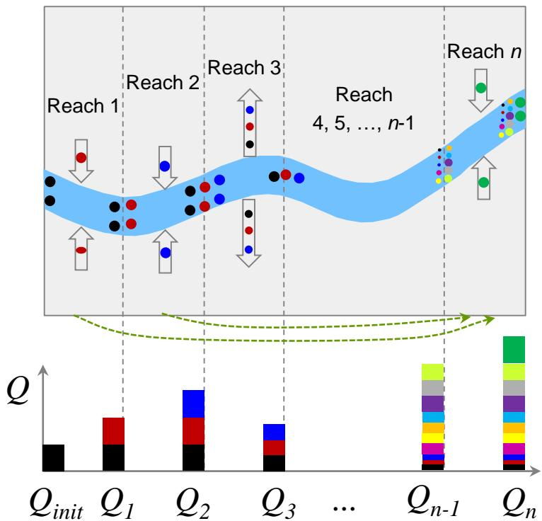
Sequential stream-groundwater exchange
