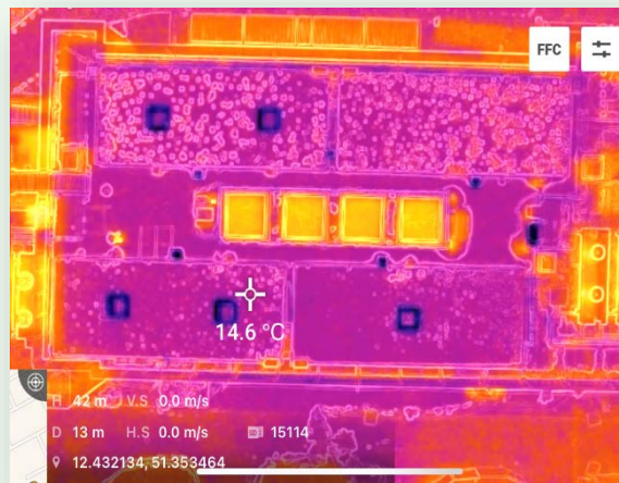
Figure: Determining surface temperature via IR camera on January 18, 2021 Author: Jan Knappe
