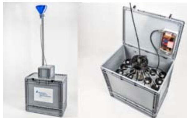
An autosampler for the sampling of rainwater
