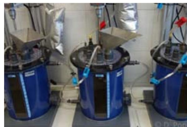
Laboratory reactors for anaerobic fermentation
