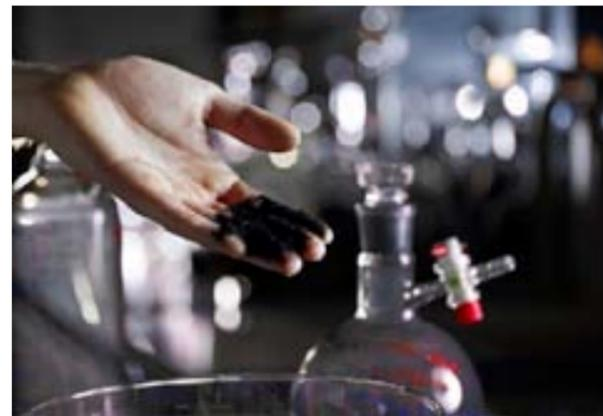
Carbo-Iron® from colloidal activated carbon and iron
