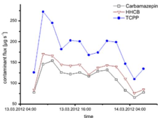
*Diurnal flux pattern of selected organic contaminants, released from a waste water treatment plant into the Ammer river.*
