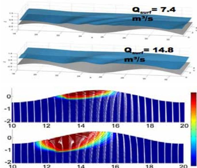
Modeled streambed geometry (upper panel) and model results (lower panel) of a 3D simulation of turbulent stream flow coupled to hyporheic flow and solute transport.
