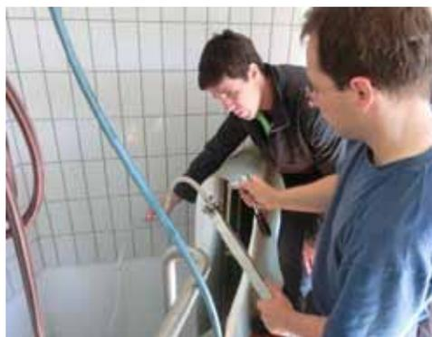
Equipotential surface from a steady-state groundwater model and flow paths to groundwater production wells (left panel). Sampling of drinking water production wells to estimate groundwater age based on environmental tracer concentrations (right panel).
