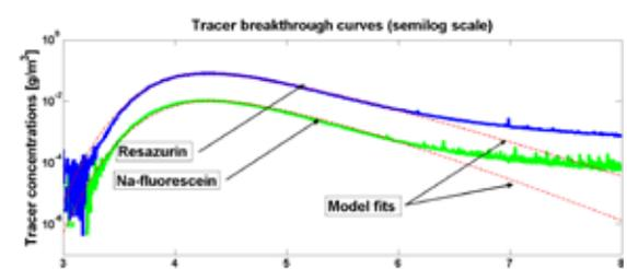
Reactive fluorescent tracer experiment and measured breakthrough curves at the Goldersbach river.
