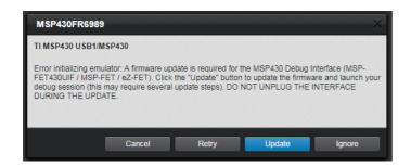
You might need to hit *run* again after such an update, if the code is not uploaded automatically. A successful upload is terminated with a message similar to "Flash/FRAM usage is 14598 bytes. RAM usage is 351 bytes."
