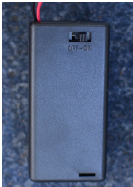
Figure 5 Switch at battery holder for power supply of logic- leave it always on or turn on first!
