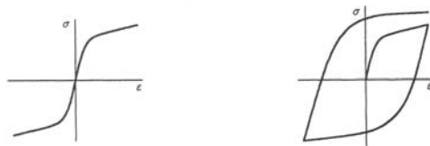
Experimentally observed rate-independent solid material behavior. Cyclic uniaxial stress-strain curves: without hysteresis (left), with hysteresis (right)
