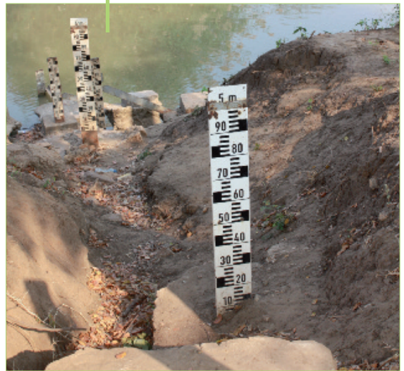
Fig.12: Water level of a river in East Africa at low water
